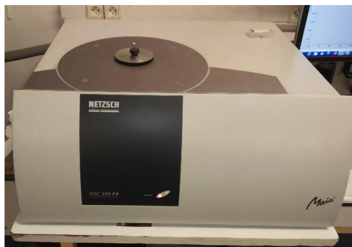
Figure 6. DSC device used to characterize the different samples.
