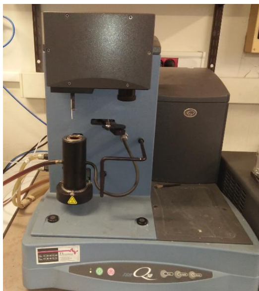
Figure 5. TGA device used to characterize the different samples.
