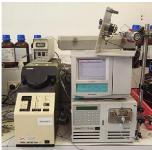
Figure 4. GPC device used to characterize the free PVDF chains extracted from the nanocomposites.
