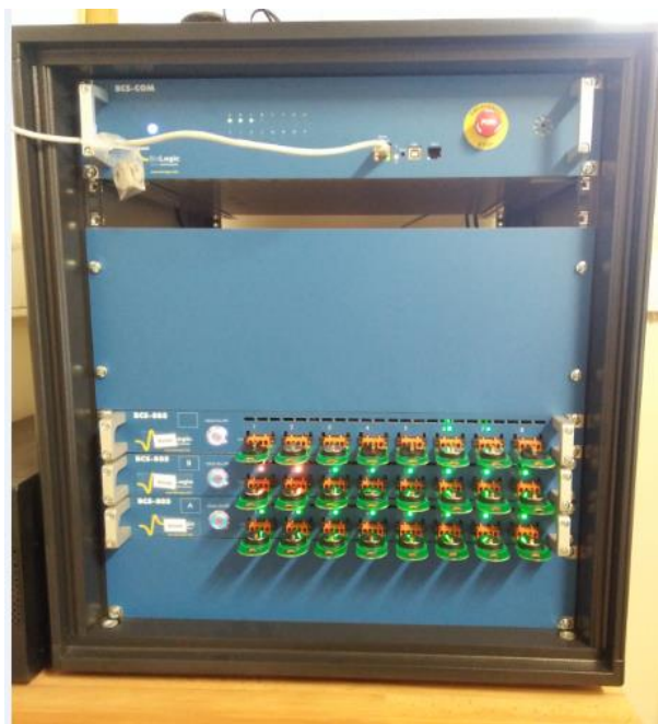
Figure 12. BCS-805 device used to perform the cycling performances of the prepared cells.
