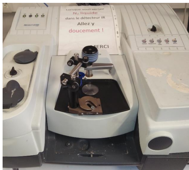
Figure 2. Picture of FTIR device used to analyze the functionalized nanoparticles and synthesized nanocomposites.
