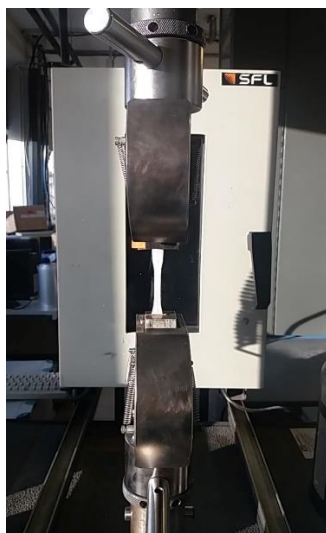
Figure 10. Tensile machine used to analyze the mechanical properties of nanocomposite films.
