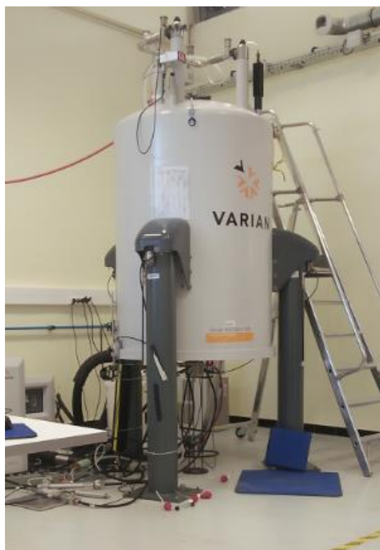
Figure 3. Picture of HRMAS NMR spectroscope used to analyze functionalized BaTiO 3 and PVDF- g -BT nanocomposites.
