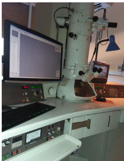
Figure 7. Transmission electronic microscope used to characterize the different samples.
