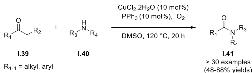
Scheme 19. Copper-catalysed amide synthesis from ketones and amines.
