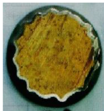
Fig. 4. Photograph of an iodine-loaded silver-silica waste form obtained by hot isostatic pressing at 750 °C and 100 MPa [73].
