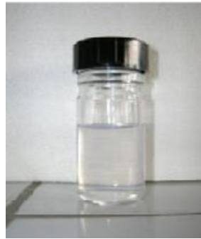
Figure 11: Example of colloidal suspension of apatite nanoparticles stabilized with AEP (Al-Kattan et al.) 37
