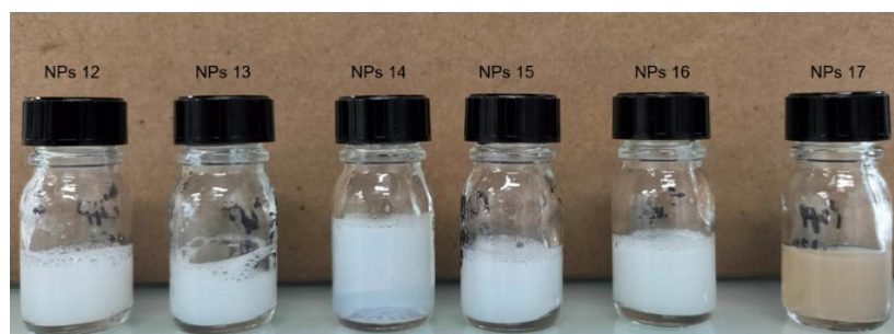
Figure 58 : Picture of colloidal suspensions obtained for different R-PO 3 H 2 /Ca starting ratios: (0.005, 0.008, 0.01, 0.016, 0.032, 0.128) giving rise to NPs 12 to 17
