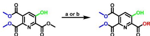
Scheme 22. Regioselective Transesterification: (a) 10 mol % EtNiPr 2 , ROH, 60 °C; (b) 5 mol % Sc(OTf) 3 , ROH, cat. H 2 O, 60 °C 208
